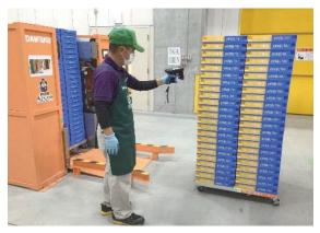
Returned foldable containers are scanned using a hand scanner.
