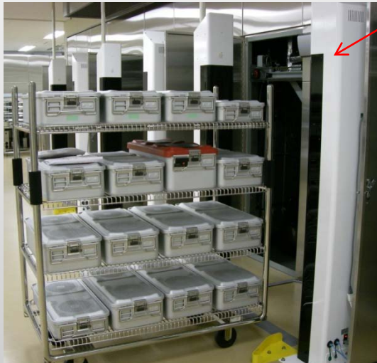
Data entry of the start of sterilization by RFID tag
