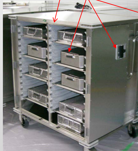
Carts for collection and RFID tags attached to inner baskets and containers
