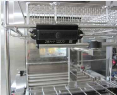
RFID tags attached to inner baskets of a cleaning machine
