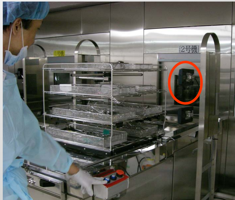
Gate-type antenna to read RFID tags for multiple tank automatic cleaning machine
