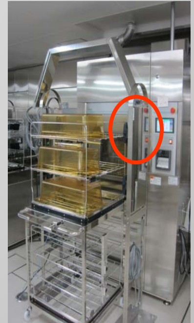
Gate-type antenna to read RFID tags for single tank automatic cleaning machine
