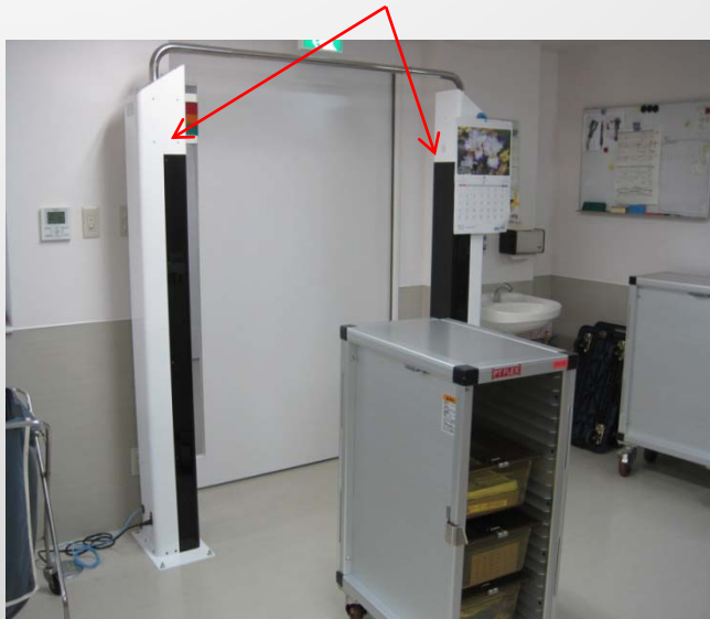
Gate-type antenna at collection points
