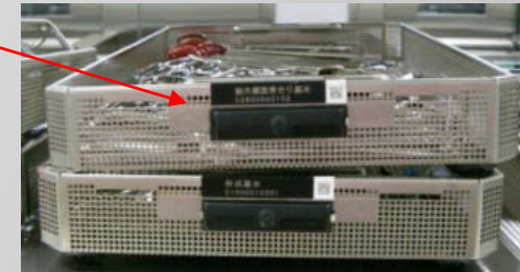
Carts for collection and RFID tags attached to inner baskets and containers
