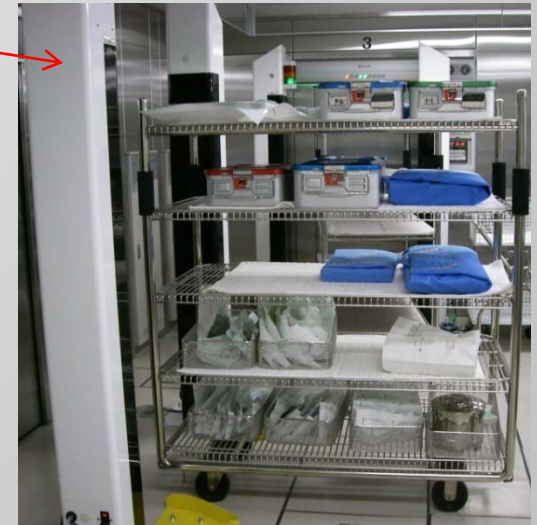
Gate-type antenna to read RFID tags for sterilization
