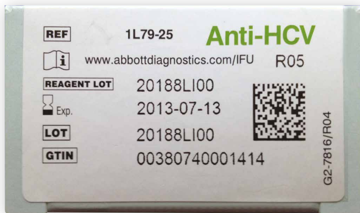
A diagnostic assay for the hepatitis C virus (anti-HCV) uses a GS1 DataMatrix bar code and a 14-digit GTIN. The expiry date uses the ISO 8601 format (YYYY-MM-DD)
