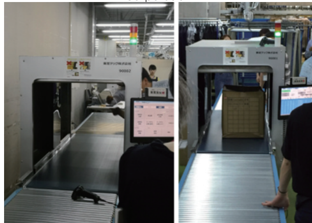
Figure 1.2.1.3-2 (3) RFID Tunnel Reader of Toshiba Tec Corporation
