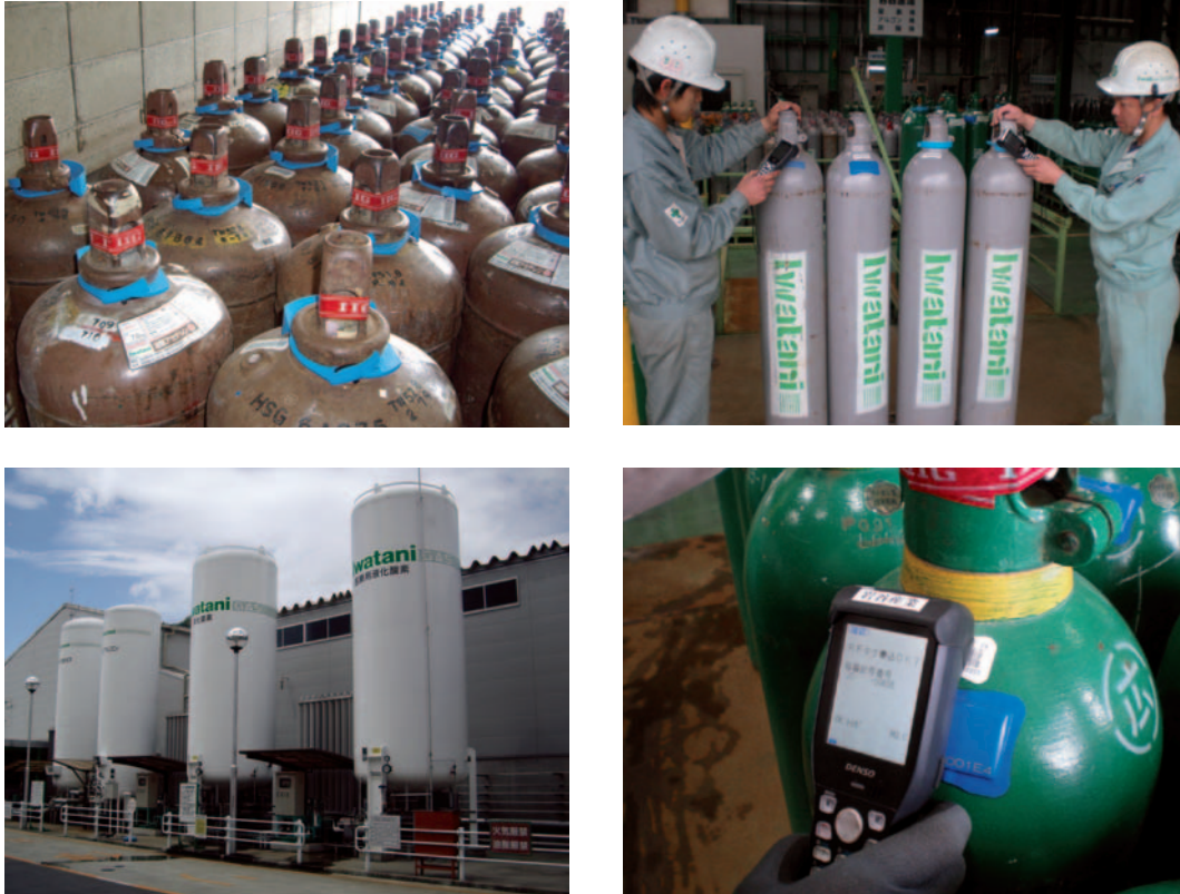
Fig. 4.3.2-1 EPC/RFID operations at a gas cylinder filling station
