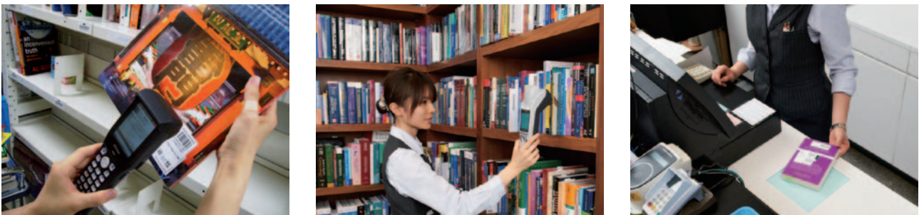
Fig. 4.3.4-2 Reading EPC tags in the bookstore (Inventory-taking and checkout at POS)
