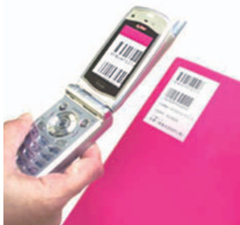
Fig. 1.3.2-2 Scanning GTIN or ISBN using cell phones with camera
