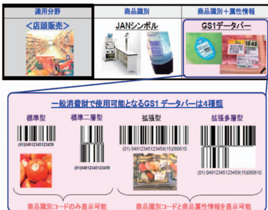
Fig. 1.6.1-1 GS1 DataBar Guideline GS1 DataBar family symbols for retail Point of Sale
