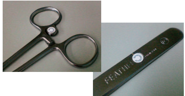
Fig. 6.2.3-3 Ceramic RFID Tags attached to medical devices
