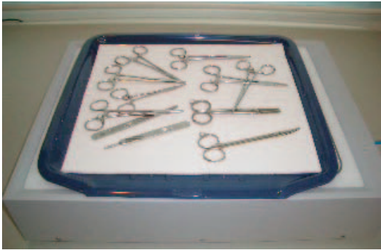
Fig. 6.2.3-2 Surgical Instruments with RFID laid on Reader/Writer
