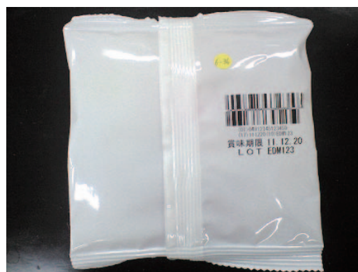
Fig. 1.5.2-2 GS1 DataBar Expanded test print with AI (01), (17) and (10)
